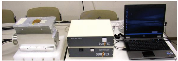
measurement head portion controller portion Lap top PC (XG power supply portion) for operation
